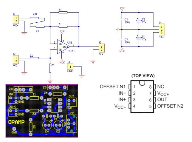
*Fig.1. Basic Operational Amplifier schematic diagram, C1-C4 capacitors are used for power decoupling; PCB of the circuit; operational amplifier TL061 – pinout;.*
